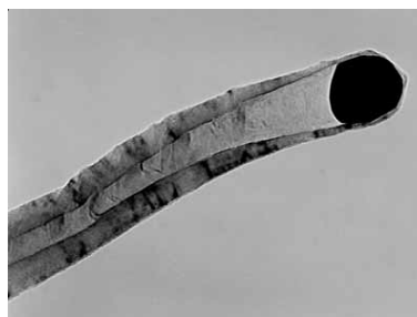
MULTIWALL CARBON NANOTUBE WITH ITS SEEDING PARTICLE (TEM)
